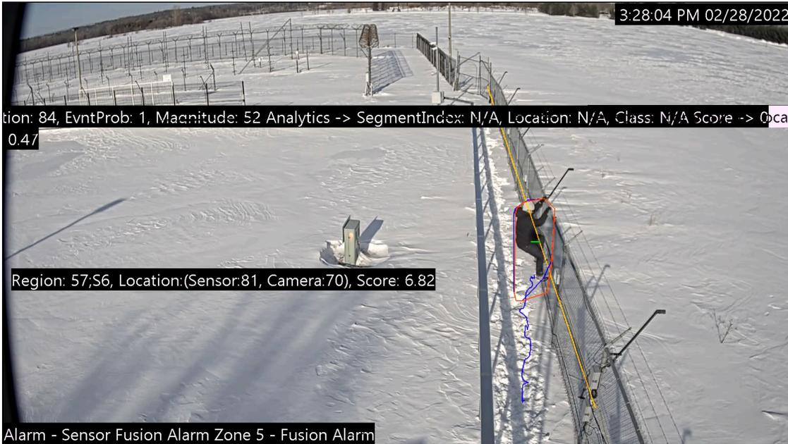
In addition, the Senstar Sensor Fusion provides redundancy if one of the components experiences a failure. When one component experiences a failure, the Senstar Sensor Fusion shifts the weight of the probability to the functional component and triggers alarms based on that probability.
