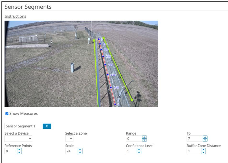
The sensor segments do not have to cover the entire perimeter intrusion detection system. The coverage of the Senstar Sensor Fusion does not depend on the perimeter intrusion detection system zone configuration; the sensor segments can be part of a single zone, part or multiple zones, or match a zone exactly.
